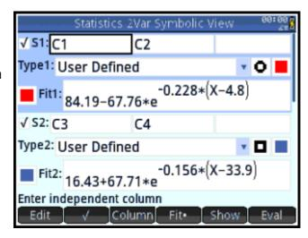
The largest difference between the empirical data and our numerical models appears at point no. 49, where the measured value amounts to 83 °C but the predicted one is 66 °C in the graph. Yet, the graph shows that the experimental data approximately follow Newton's law of warming and cooling.
